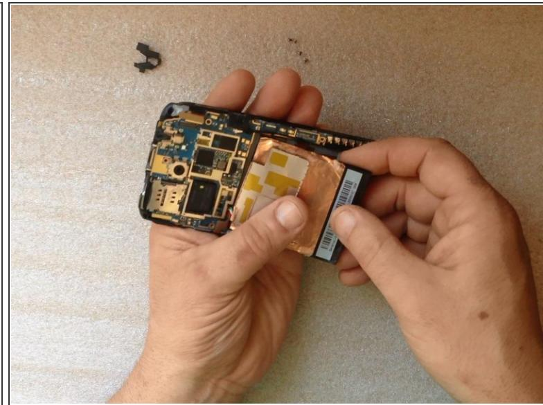
*(i)* A piece of copper tape covers the battery and an EMI shield on the motherboard.
